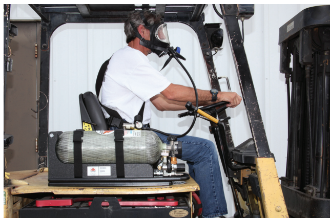
PAK-SFL™ & bracket mounted on forklift
